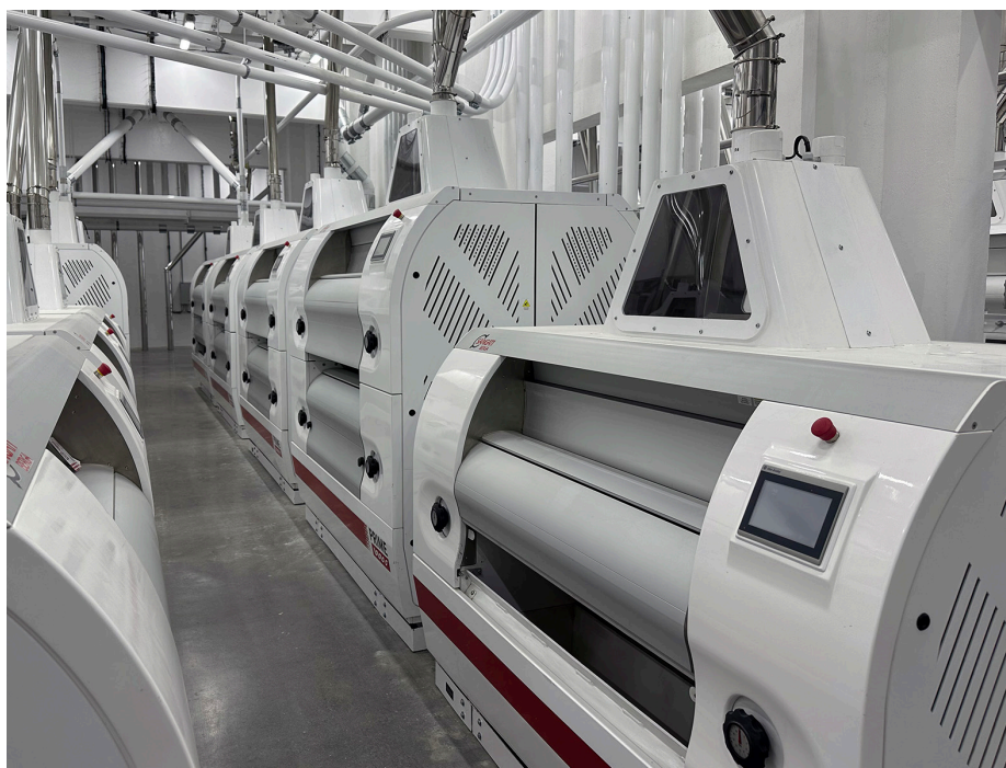
GRIND AND SIFT: Amber Wave's flour mill produces just under 3 million pounds of flour each day. The mill's roll grinders and sifters are from Sangati, one of the top producers of milling equipment worldwide; The milling process extracts the endosperm, which becomes the flour, and peels off the outer layer of the wheat kernel, also known as bran or wheat midds.
